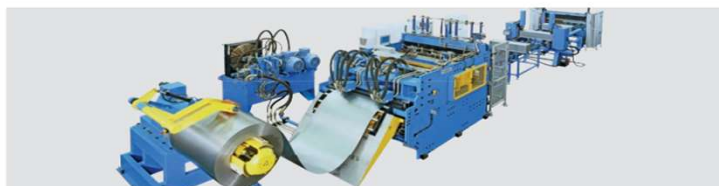
Corrugated fin panel production line type TFF5 1600-400
